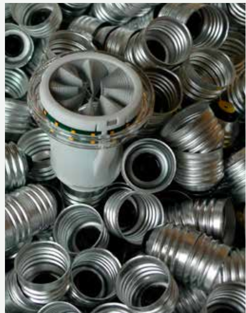
AT Lighting has 3D-printed an aluminium cooler core with a powerful 2000 lumen LED module as a part of the HYPERCOOL project funded by Innovation Fund Denmark. The cooler core will be a visible part of the finished lamp. Two prototypes of AT Lighting’s CoolLED bulb from the EUDP CoolLED project on a “bed” of old E27 fittings.
